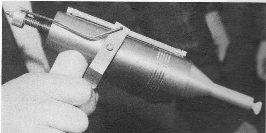
Below: the Serpent 'pistol-grip' fuel filler will re-fill a tank in a split second. With this item, plus the quick-change wheels, the Serpent team are able to attain low pit-stop times comparable with Brabham's full-size pit crew.
