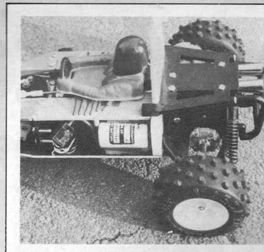
Right: the rear suspension and drive universal joints should be carefully assembled and checked over periodically to ensure trouble-free operation.
