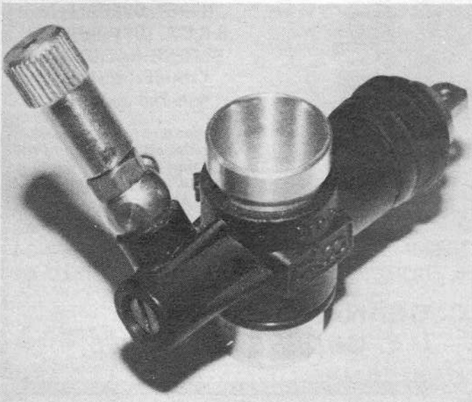
Below left: the latest Picco slide carburettor now features a moulded plastic body plus all the usual handy features. Below right: the updated Serpent rear wheel fixing, now incorporating a quick change system, very similar to the SG and PB versions. A new rear wheel hub has also been specially moulded to complement the new fixing.
