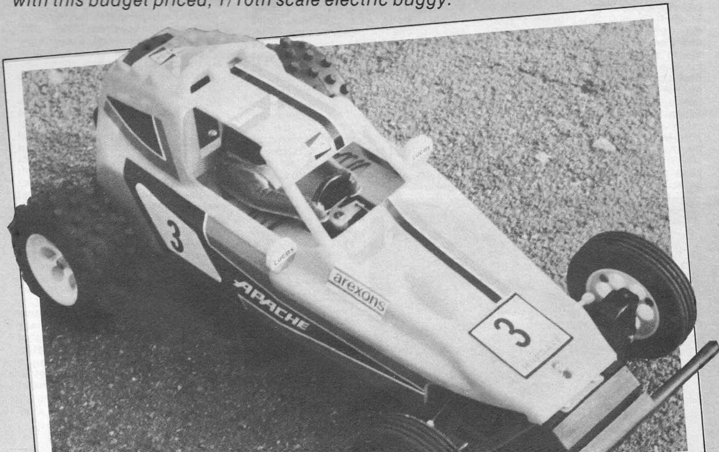
Above: the completed 'Apache' chassis goes together to form a very robust and rigid structure. Note: some thread-lock should be applied to the speed controller disc nut to stop it vibrating loose.
